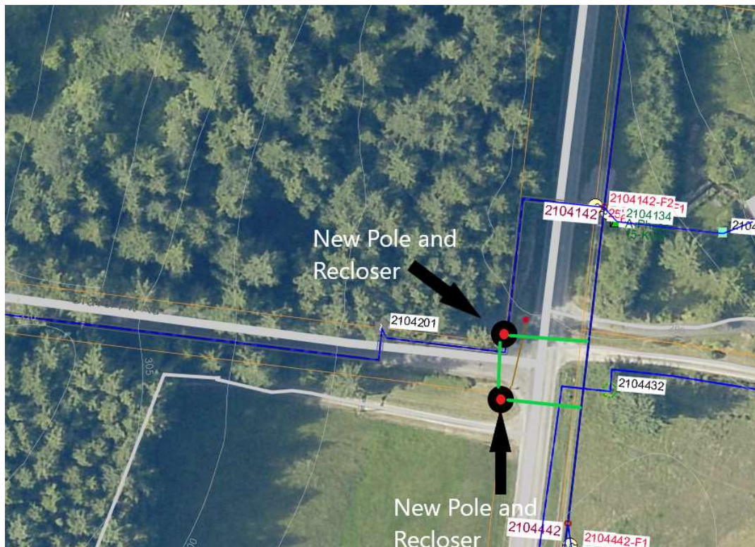
Figure 1: Overhead Construction Overview
