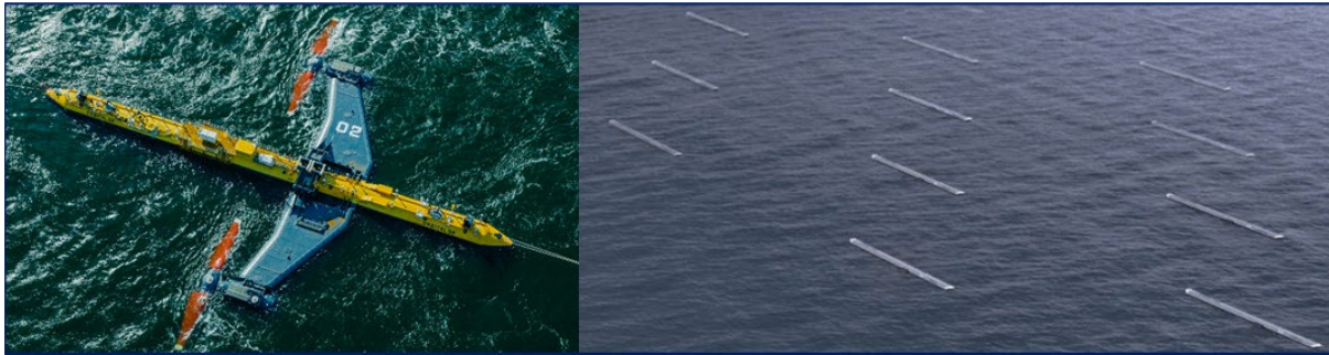
Figure 4. Orbital O2 2MW tidal turbine (delivered under H2020 FloTEC GA. 691916) and O2 tidal farm illustration.
