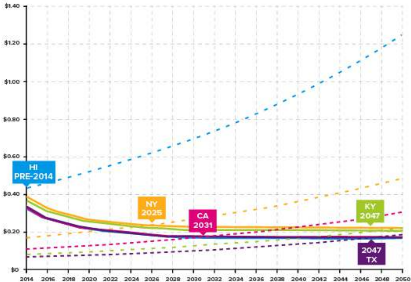
SOLAR-PLUS-BATTERY LEVELIZED COST OF ELECTRICITY (LCOE) VS. UTILITY RETAIL PRICE PROJECTIONS COMMERCIAL - BASE CASE [Y-AXIS $/kWh]
